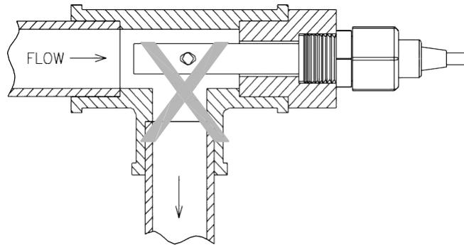
The measurement error or instability can be caused by the flow cannot guarantee the full pipe or high gas accumulation.
