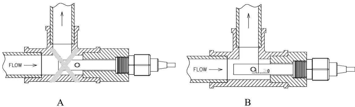
2) The installation mode of A will lead to the formation of the air cavity in the conductivity cell, resulting in measurement errors and instability, and should be installed as shown in figure B.
