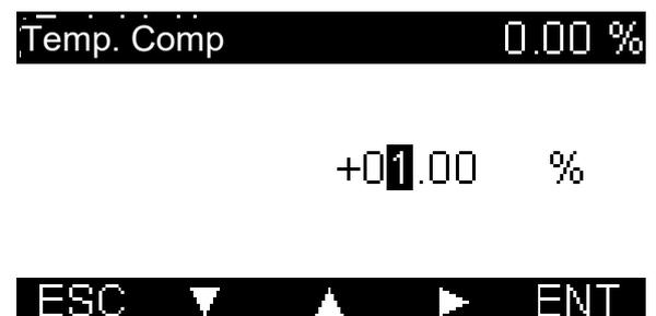
parameter according to the actual situation. After pressing the Enter key to confirm, the measured value will change according to the temperature compensation parameter.
